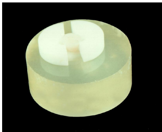
Figure 1: The Test Specimen with polytetrafluoroethylene inverted cone mold
