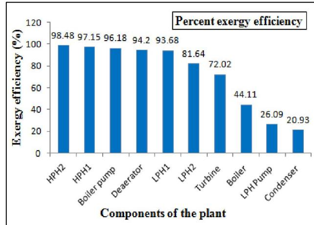
**Figure 2:** (a) Exergy destruction, (b) Exergy efficiency of every components of the plant
