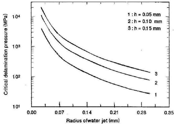
Figure (3): Critical delamination pressure versus radius of water jet at different values of uncut thickness.
