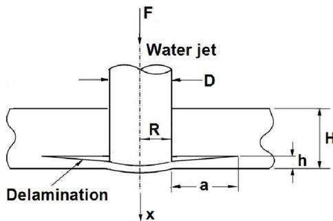
Figure (1): A schematic drawing for the circular plate model of delamination fracture analysis.
