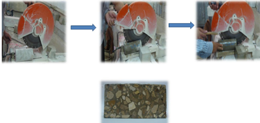
Photo (1): Preparing the longitudinal sections
