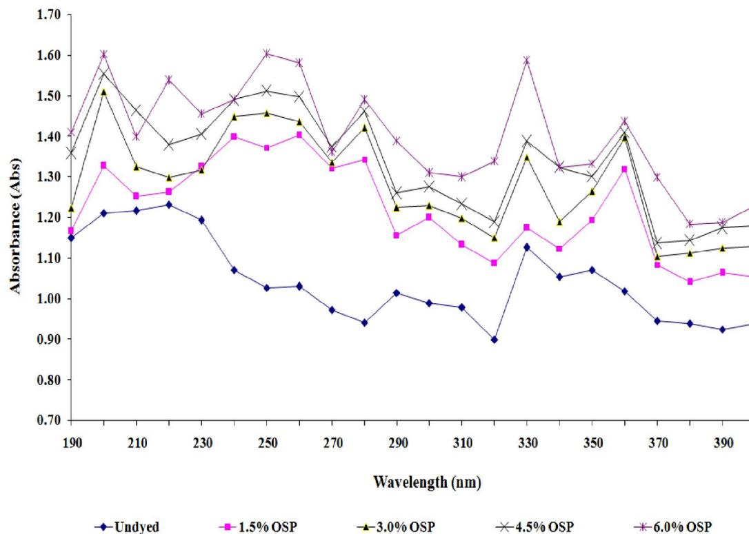
**Figure 3.** Ultraviolet absorption (Abs) of cotton fabric dyed with different onion skin extract dye concentrations and using 10g/L  $\text{CuSO}_4$  as a mordant
