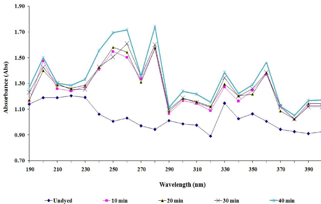
**Figure 2.** Ultraviolet absorption (Abs) of cotton fabric dyed with 4.5 g/L onion skin extract dye solution and using 10 g/L  $\text{CuSO}_4$  mordant for different times
