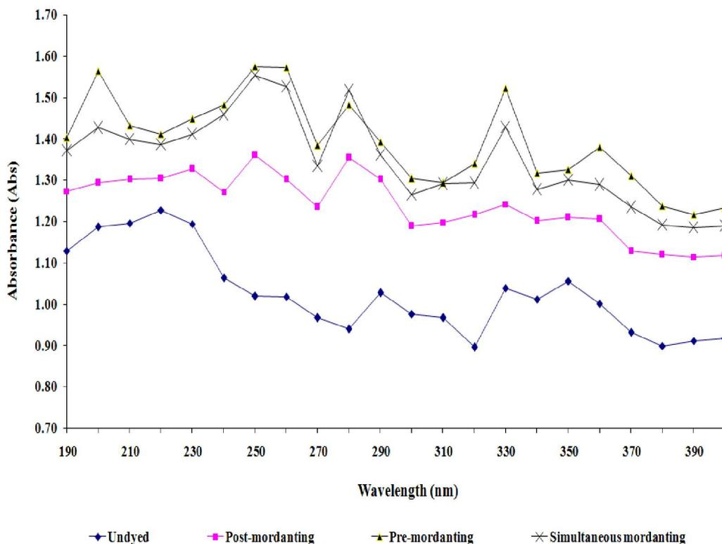
**Figure 5.** Ultraviolet absorption (Abs) of cotton fabric dyed with 4.5 g/L onion skin extract dye solution and using 10 g/L  $\text{CuSO}_4$  mordant by pre-, simultaneous and post mordanting techniques
