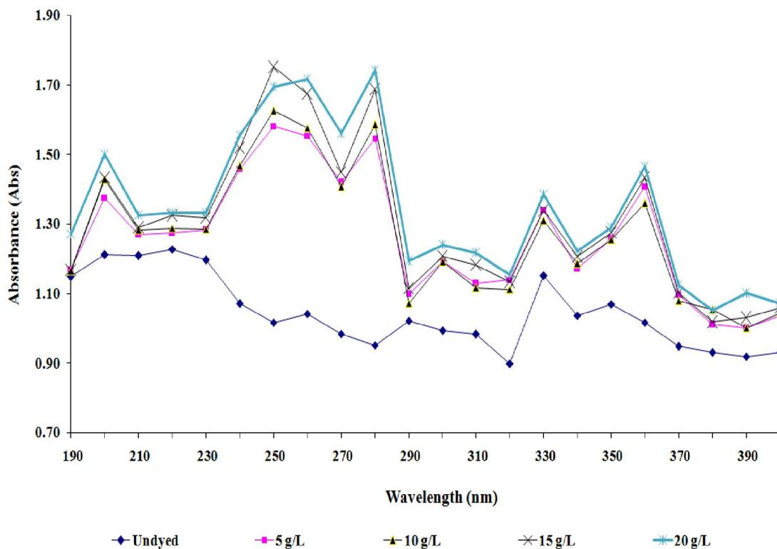
**Figure 1.** Ultraviolet absorption (Abs) of cotton fabric dyed with 4.5 g/L onion skin extract dye solution and using different concentration of  $\text{CuSO}_4$  mordant
