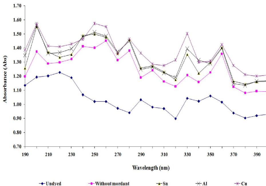
**Figure (4).** Ultraviolet absorption (Abs) of cotton fabric dyed with 4.5 g/L onion skin extract dye solution and using 10g/L mordant
