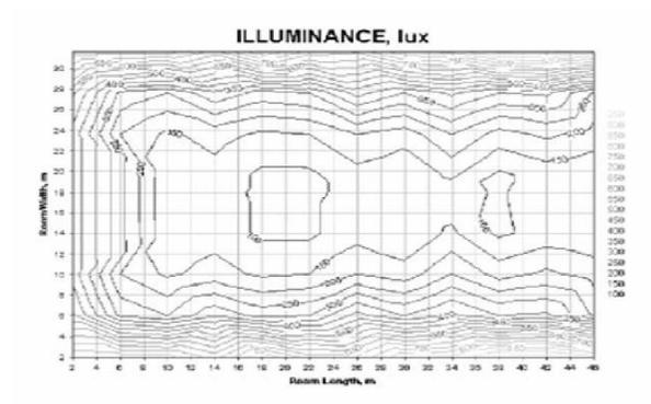
Figure 7. Measured illumination (lux) in the simulation model of the hall.
