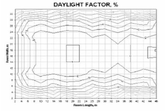
Figure 5. DF contour lines as measured in the simulation model of the hall and location of measured points
