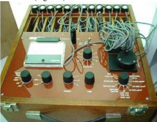
Figure 4. Daylighting factor meter
