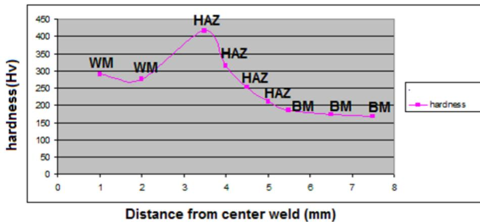
**Fig.11** Hardness distributions along weld metal, HAZ and base metal using E7018 electrode and applying a heat input of 0.89 kJ/mm without preheating
