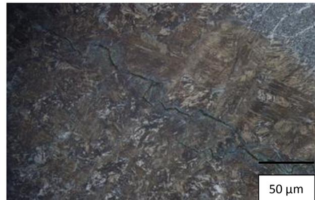
**Fig. 9** Microstructure at the cracked HAZ
