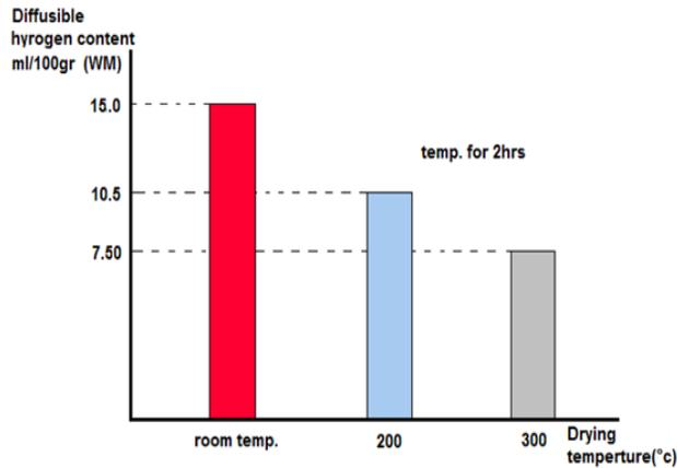
**Fig. 2** The effect of drying temperature on the diffusible hydrogen content
