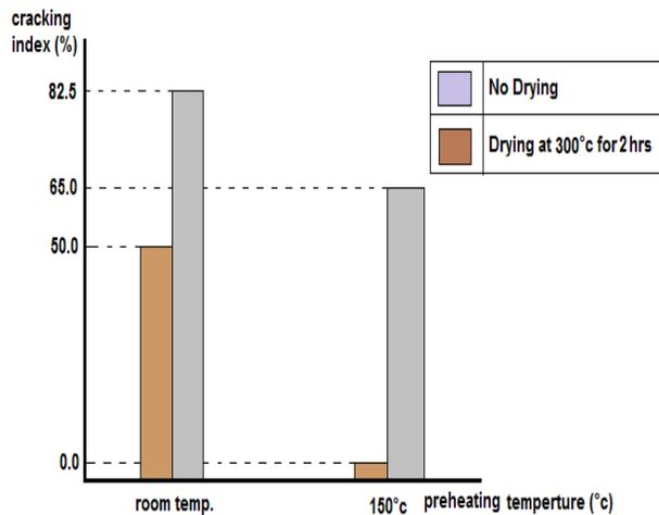
**Fig. 3** Effect of preheating temperature on cold cracking index
