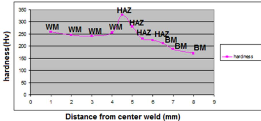
Fig. 12 Hardness distributions along weld metal, HAZ and base metal using E7018 electrode and applying a heat input of 0.89 kJ/mm with preheating temperature of 150 °C
