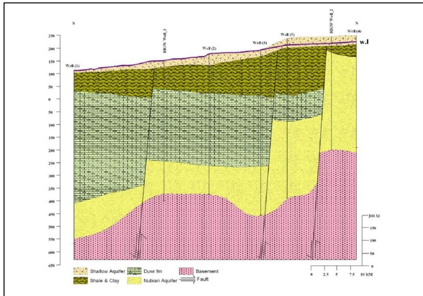
**Figure 2. Aquifer configuration of Wadi Qena**
