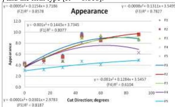
Figure (11): Appearance for seamed fused fabric
