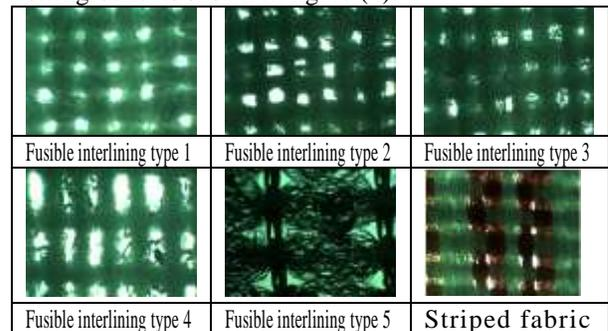
Figure (4): Fluorescence microscopic pictures for striped fabric and all types of fusible interlining
