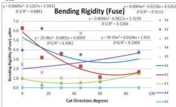
Figure (7): Bending Rigidity for fusible interlining
