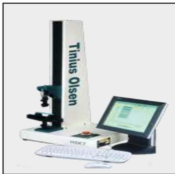
Figure (6): Tinius Olsen tensile strength and elongation tester
