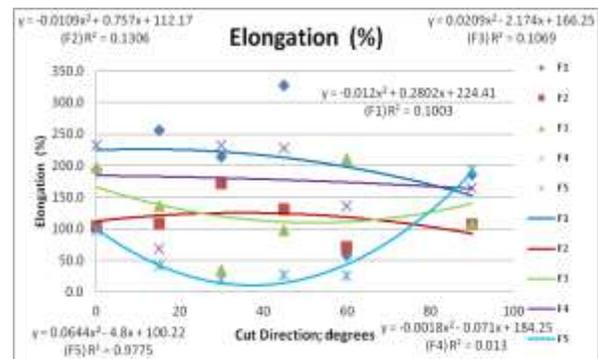
Figure (10): Elongation for seamed fused fabric
