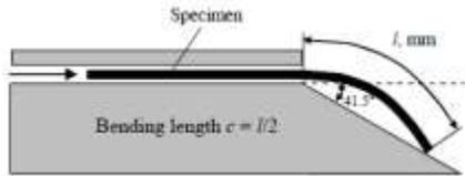
Figure (5): Specimen bending in FAST system
