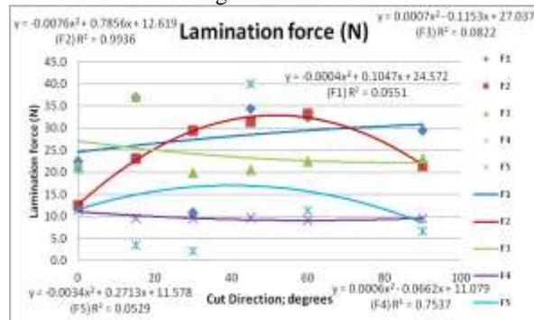
Figure (9): Lamination force for seamed fused fabric
