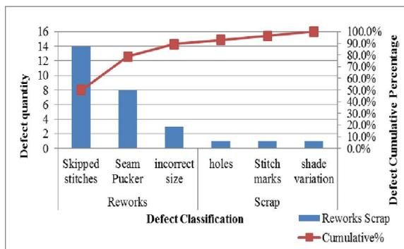
Figure (9). Pareto diagram for sewing defects
