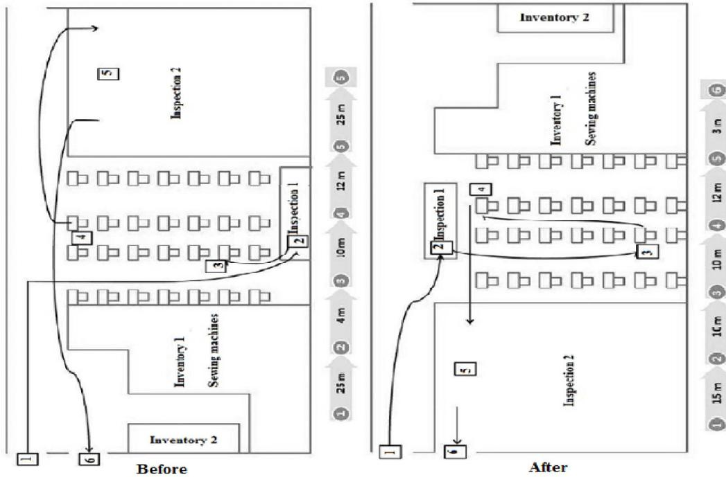
Figure (1): Spaghetti diagram for sewing section before and after applying lean principles
