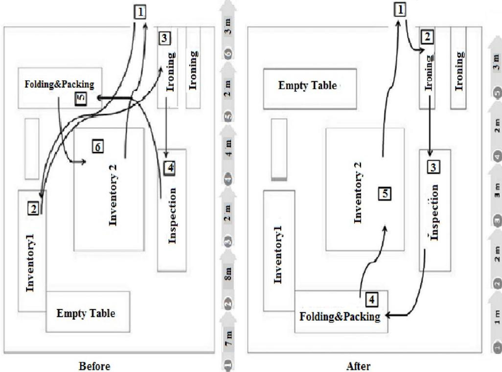
Figure(2): Spaghetti diagram for packing section before and after applying lean principles.
