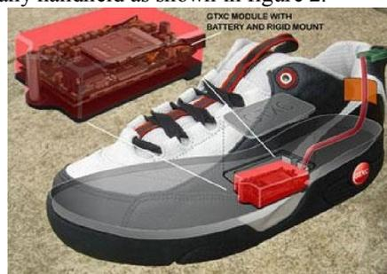
Figure 2. showing the tracking shoe
