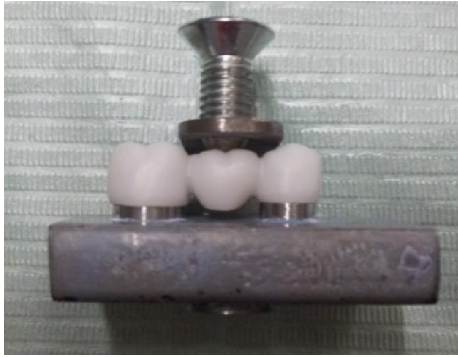
(Figure 7): The bridge held on the master model using specially fabricated design
