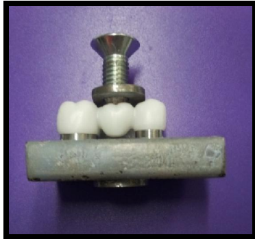
(Figure 5): A sample secured on the specially fabricated holding device.
