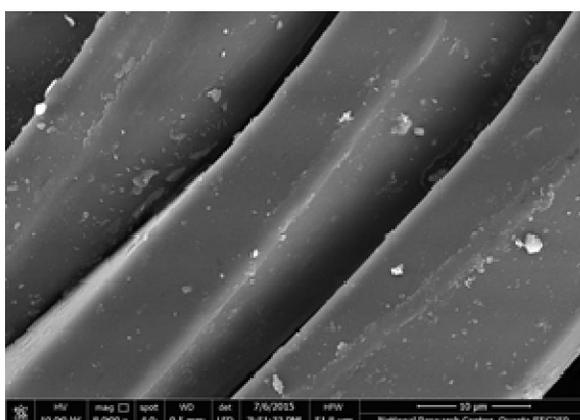
Figure 7: SEM of Plasma O<sub>2</sub> treated (8mA for 5min) F1
