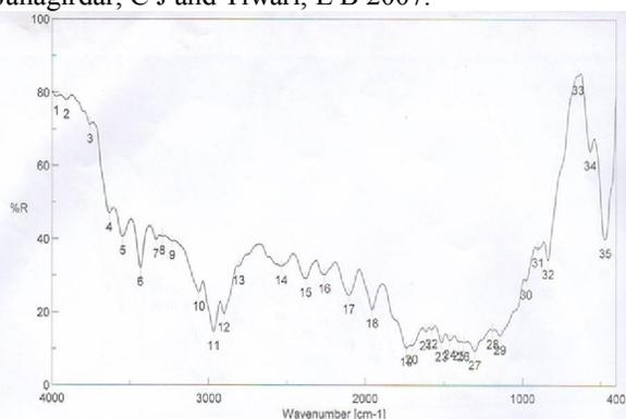
Figure 3: FTIR Spectrum of Untreated Warp PET
