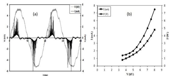
Figure (2) a: current – voltage waveforms of the discharge produced in air and b: variation of the discharge current and power with applied voltage for DBD air discharge
