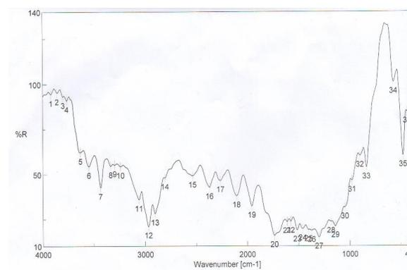
Figure 5: FTIR Spectrum of Plasma Air treated Warp PET
