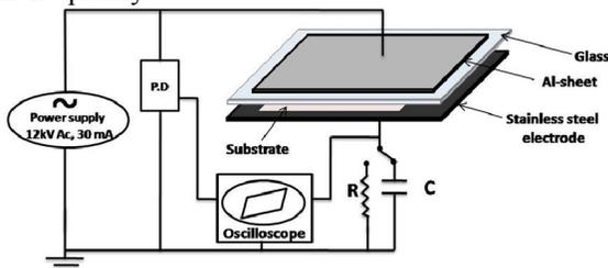
Figure (1) schematic diagram of DBD cell used for treatment of the fabrics
