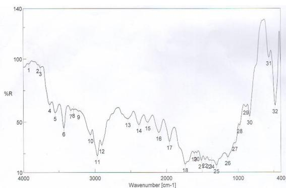
Figure 4: FTIR Spectrum of Plasma Oxygen treated Warp PET
