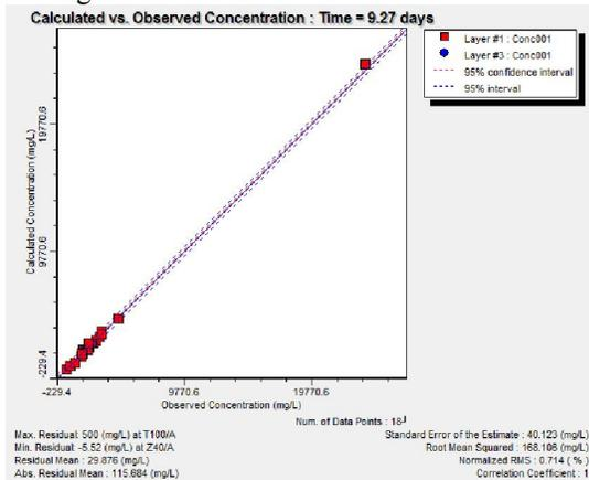
**Fig.(9) Steady state calibration results (TDS)**
