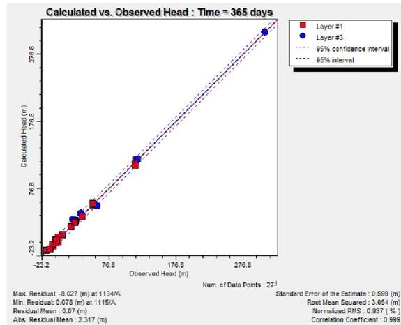
**Figure (8): Steady state calibration results (head)**
