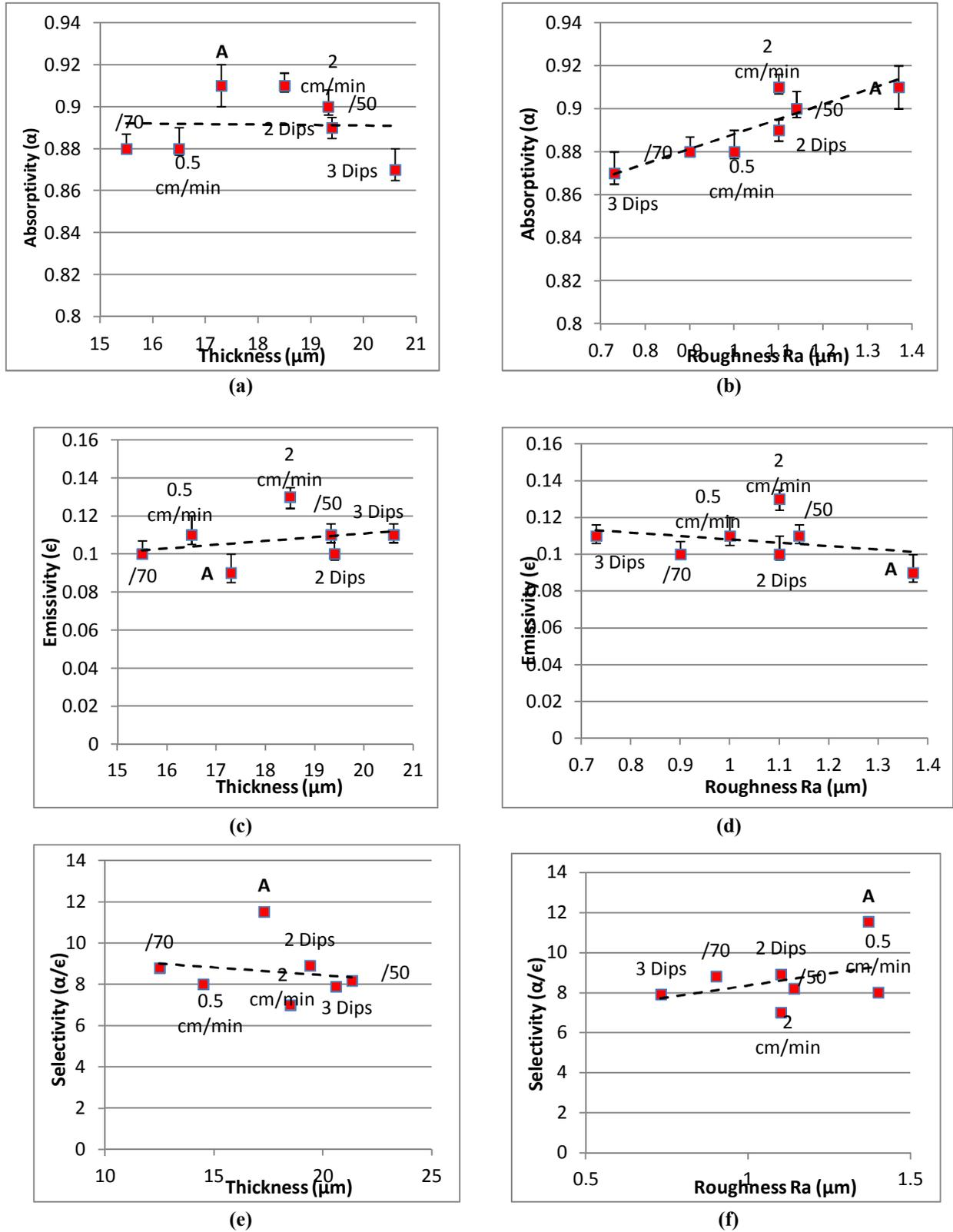
Fig. 8: Effect of thickness and roughness on (a), (b) absorptivity, (c), (d) emissivity, (e), (f) Selectivity, where A is the best selectivity of molar ratio /60 1 cm / min and 1 dip.
