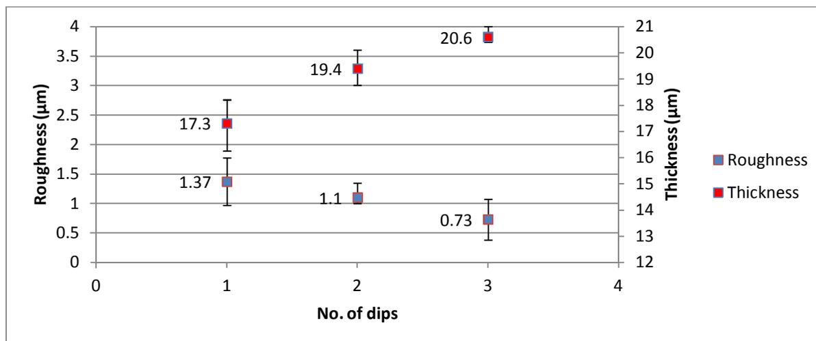
**Figure 6: Thickness and roughness versus number of dips relation for stainless steel samples coated**
