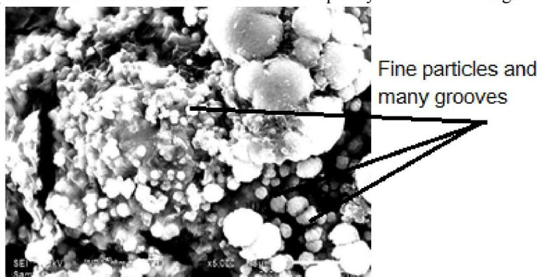
**Fig. 4: SEM of Stainless steel sample coated with  $\text{CuCoMnO}_x$  with highest selectivity 10.11, absorptivity 0.91 and emissivity 0.09. Preparation conditions: molar ratio /60 and withdrawal rate is 1 cm/min and only one dip in the coat. Magnification X 5000**
