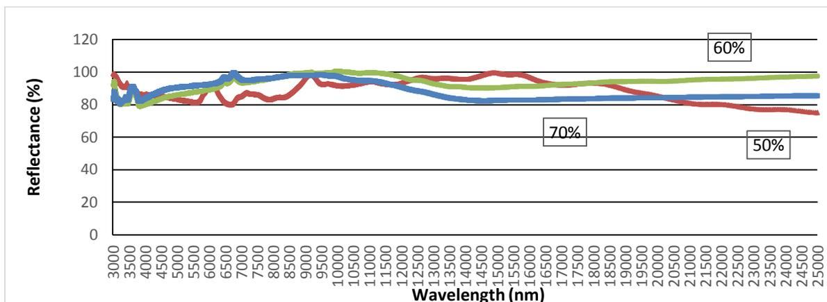
Fig. 3: Reflectance measurements in IR range for measuring emissivity of Stainless steel samples after the dipping-heat treatment cycle, in three different solutions with molar ratio of chemicals /50 (molar 50), /60 (molar 60) and /70 (molar 70).
