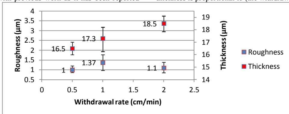
**Fig. 5: Effect of withdrawal rate on the thickness and roughness of the coated samples.**
