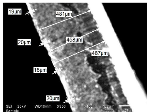
Fig. 1: Thickness of the samples measured by the SEM microscope
