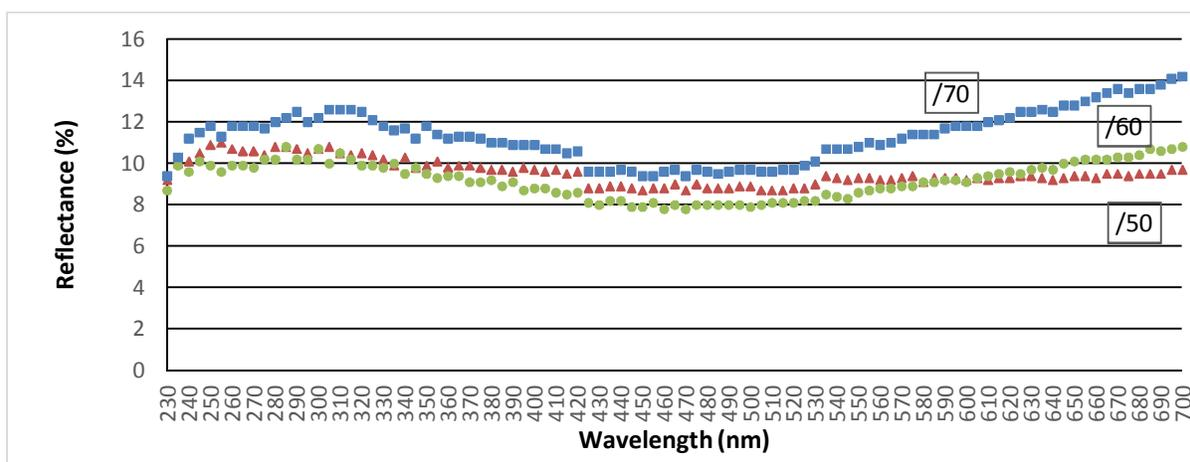
Fig. 2: Reflectance measurements in UV range for measuring absorptivity of Stainless steel samples after the dipping-heat treatment cycle, in three different solutions: with molar ratio /50 (molar 50), /60 (molar 60) and /70 (molar 70).
