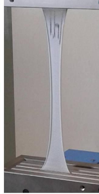
Fig.5. Snarling of single Jersey edge during tensile test.
