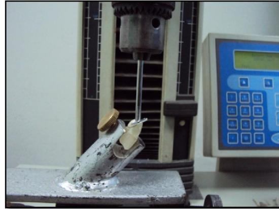
**Figure 5:** lateral loading (proximal view)
