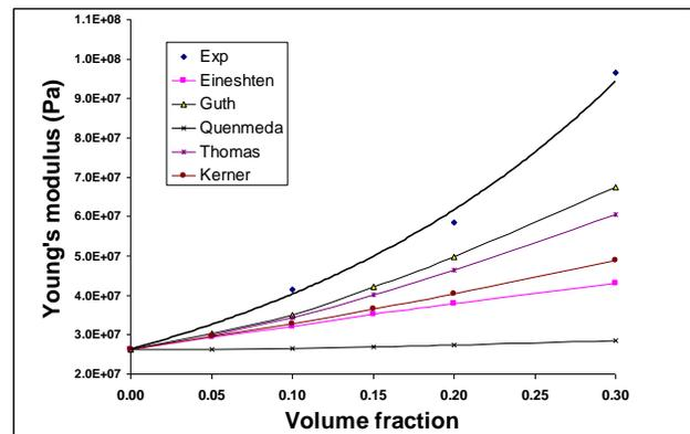
**Figure (3.5): The relation between Young's modulus and volume fraction of PPY concentration (phr) with the theoretical models for all samples.**
