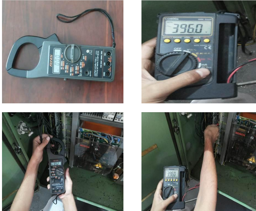
Fig.4 Avometer and clip ampere which had been used to measure voltage and amperage used in FSW welding.
