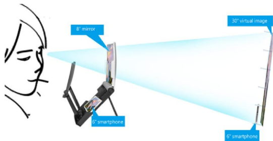
Fig. 9. Using the combination of a convex and a concave mirror with the folding mechanisms.
