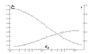
Fig.4 The respectively corresponding relationship of  $E_d/E_{dmax} \cdot \lambda_d$  and  $\epsilon_d$  in upstream sanded shell Table5 Approximation parameter of elastic modulus damp ratio
