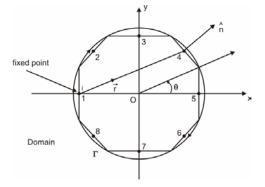
Figure 2. Discretization of the circular cylinder into 8 constant boundary elements
