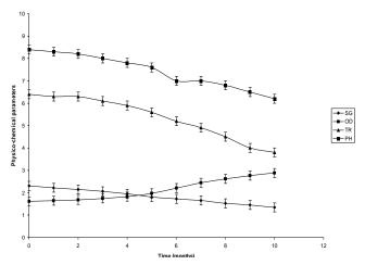
Figure 2. Mean changes in the physico-chemical parameters in fresh paint samples PS1 - PS6. SG, specific gravity; OD, 600 nm; TR, transmittance. Data represent the averages of triplicate determinations.
