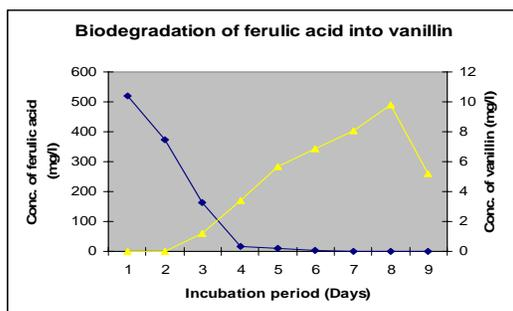
Figure 1. Time course degradation of ferulic acid and subsequent formation of vanillin by *Staphylococcus aureus* (Without glucose)
