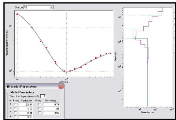
Figure: 2 Sample of resistivity field curves
