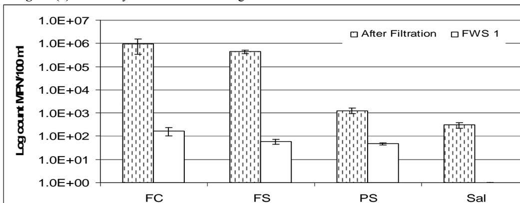
Figure (6) Efficiency of FWS 1 with triangular water entrance for the removal of some selected bacteriological strains.
