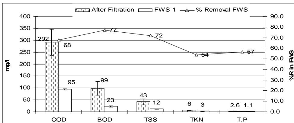
Figure (5) Efficiency of FWS 1 with triangular water entrance for the treatment of wastewater.
