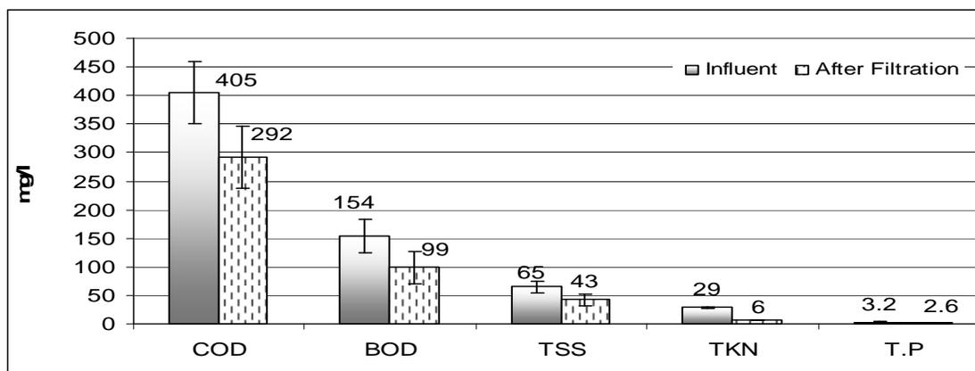
**Figure (3)** Efficiency of filtration process for the removal of COD, BOD, TSS, TKN and TP.
