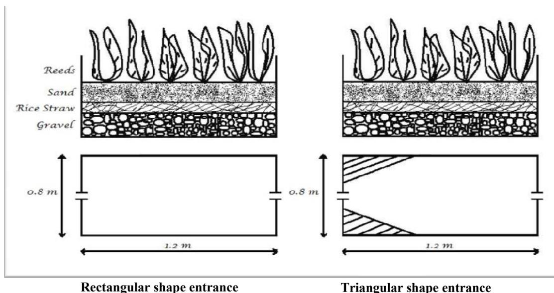
**Figure 1:** Schematic diagrams for the dimensions of the wetland system.
