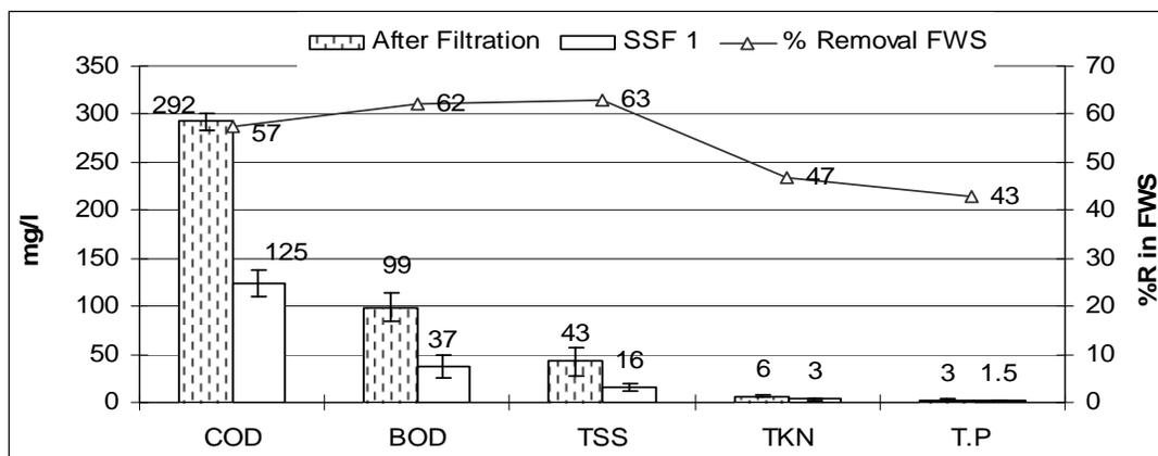
Figure (9) Efficiency of FWS with triangular water entrance for the treatment of wastewater.
