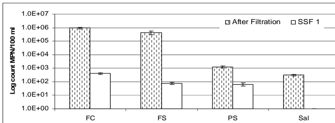
Figure (10) Efficiency of FWS with triangular water entrance for the removal of some selected bacteriological indicators.
