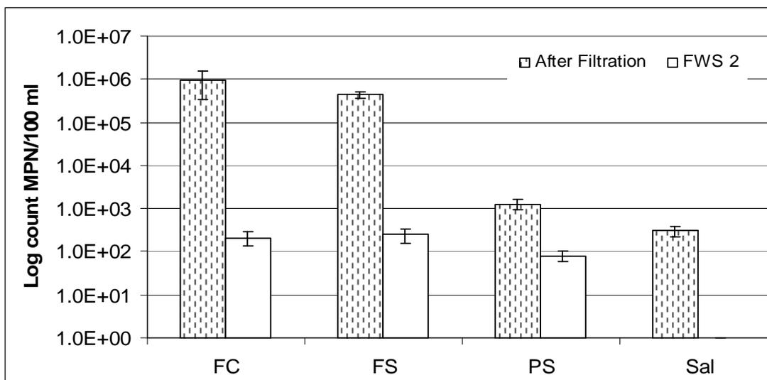
**Figure (8)** Efficiency of FWS 2 with triangular water entrance for the removal of some selected bacteriological strains.
