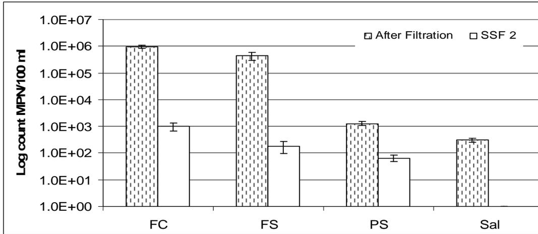
Figure (12) Efficiency of FWS with triangular water entrance for the removal of some selected bacteriological indicators.
