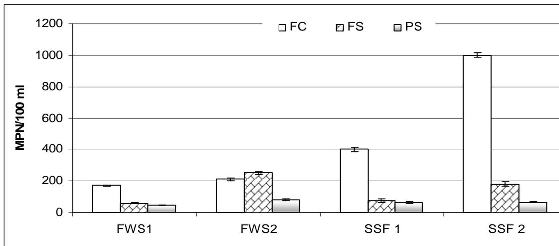
**Figure (14)** Efficiency of wetland systems for removal of indicator bacteria.
