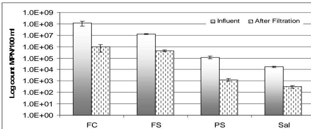
Figure (4) Efficiency of filtration process for the removal of FC, FS, PS and Salmonella.
