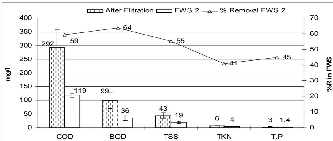
**Figure (7)** Efficiency of FWS 2 with triangular water entrance for the treatment of wastewater.
