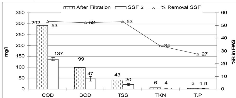
Figure (11) Efficiency of FWS with triangular water entrance for the treatment of wastewater.
