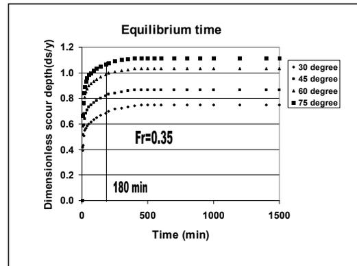
Figure3. Equilibrium time in the different position for a T-shape spur dike
