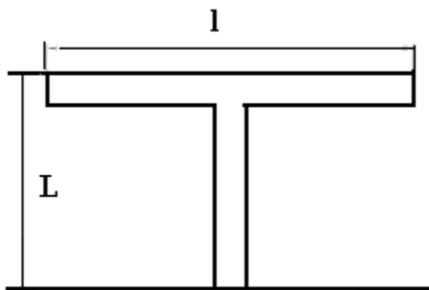
Figure2. A T-shape spur dike (Plan)
