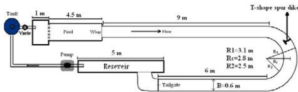
Figure1. The experimental setup (Plan)
