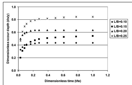
Figure7. Time development of scour for different lengths
