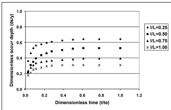
Figure9. Time development of scour for different wing lengths
