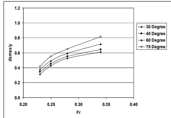
Figure6. Effect of Froude number on relative maximum depth of scour
