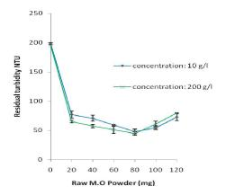
Figure 2: Average residual turbidity after coagulation with the MOC-DW solution of 10 g/l and 200 concentrations
