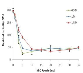
Figure 4: Average residual turbidity after coagulation with the MOC-SC solution of 200 g/l concentration
