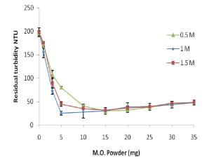
Figure 3: Average residual turbidity after coagulation with the MOC-SC solution of 10 g/l concentration
