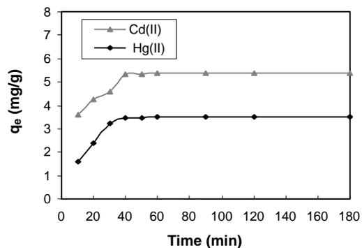
Fig. 5. Effect of contact time on the adsorption of cadmium (II) and mercury (II) by rice husk ash.  $T = 25^\circ\text{C}$ ,  $t = 6\text{ hr}$ ,  $C_0 = 100\text{ mg/l}$ , and  $m = 10\text{ g/l}$
