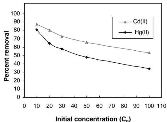
Fig. 4. Effect of the initial metal ion concentration on the removal of cadmium (II) and mercury (II) by rice husk ash.  $T = 25^\circ\text{C}$ ,  $t = 6\text{ hr}$ ,  $pH = 6$ , and  $m = 10\text{ g/l}$ .
