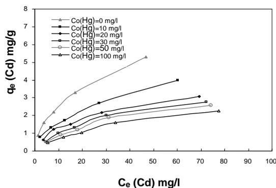
Fig. 6. Comparison of the equilibrium adsorption of cadmium (II) ion at varying concentrations of mercury (II) ion.  $pH_0 = 6$ ,  $t = 6\text{ hr}$ ,  $T = 25^\circ\text{C}$ ,  $C_0[\text{Cd(II)}] = 10\text{--}100\text{ mg/l}$ , and rice husk ash dosage =  $10\text{ g/l}$ .
