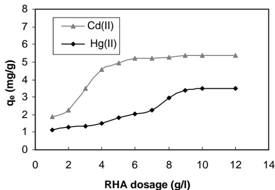
Fig. 3. Effect of rice husk ash (RHA) dosage on the removal of cadmium (II) and mercury (II).  $T = 25^\circ\text{C}$ ,  $t = 6\text{ hr}$  and  $C_0 = 100\text{ mg/l}$ .
