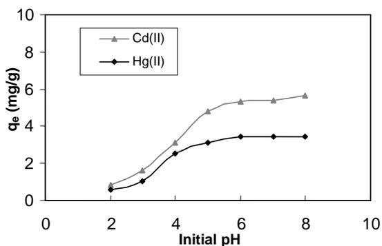
Fig. 2. Effect of  $pH_0$  on the removal of cadmium (II) and mercury (II) ions for mono-component adsorbate aqueous solution by rice husk ash.  $T = 25^\circ\text{C}$ ,  $t = 6\text{ hr}$ ,  $C_0 = 100\text{ mg/l}$ , and  $m = 10\text{ g/l}$ .
