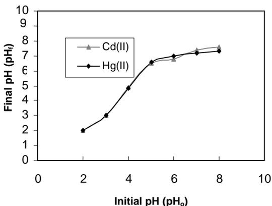
Fig. 1. The variation in equilibrium system  $pH_f$  with  $pH_0$  during the sorption of Cd(II) and Hg(II) onto rice husk ash
