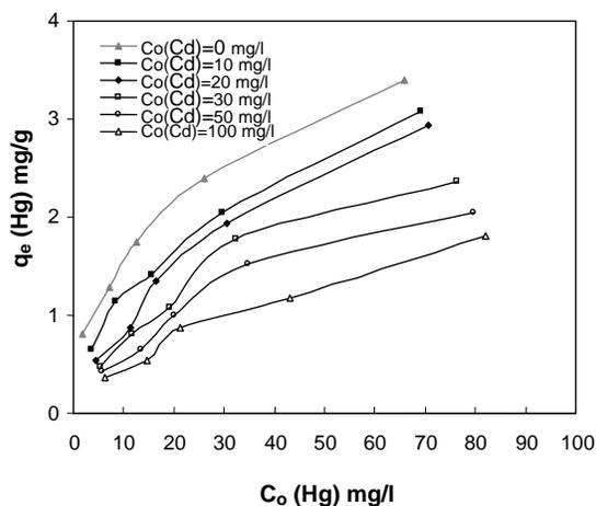
Fig. 7. Comparison of the equilibrium adsorption of mercury (II) ion at varying concentrations of cadmium (II) ion.  $pH_0 = 6$ ,  $t = 6$  hr,  $T = 25$  °C,  $C_0[\text{Hg(II)}] = 10\text{-}100$  mg/l, and rice husk ash dosage = 10 g/l.
