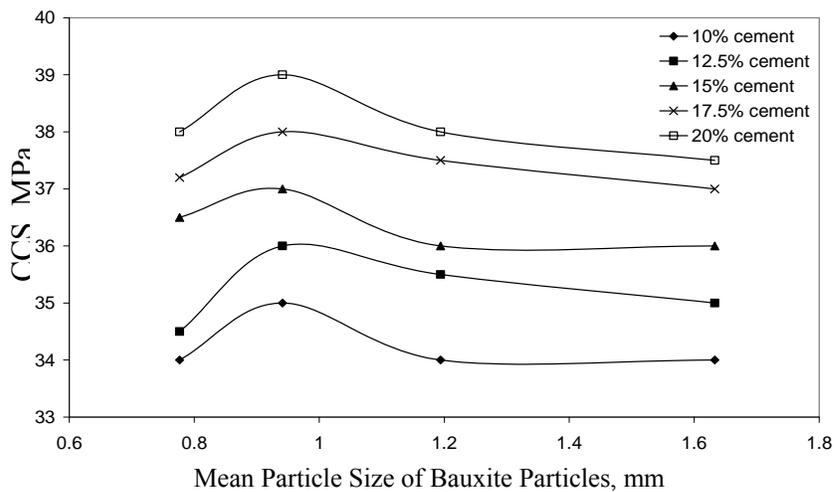
**Fig. (12): Effect of Mean Particle Size of Bauxite Aggregates Containing Different Cement Percents on the Cold Crushing Strength of Mixes**
