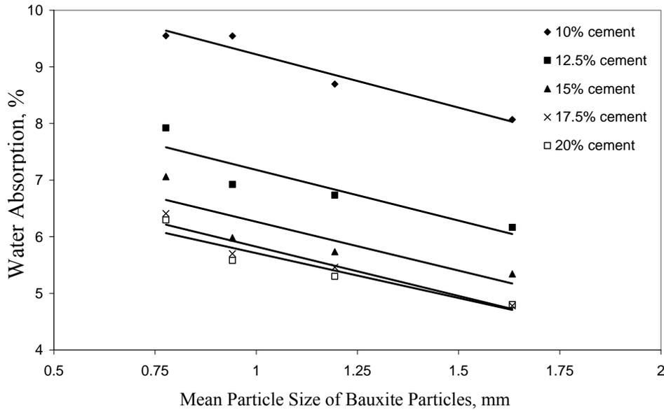
**Fig. (6): Effect of Mean Particle Size of Bauxite Aggregates Containing Different Cement Percents on Percent Water Absorption for Mixes**
