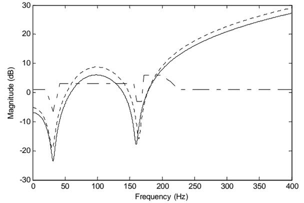
Figure 5: Output sensitivity constraint (dashed-dot) and the inverse of the Output sensitivity weighting function of  $H_\infty$  Controller (dotted) and the inverse of the Output sensitivity weighting function of  $H_2$  Controller (solid)
