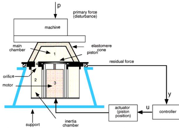
Figure 1. Schematic diagram of the active suspension system
