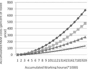
Figure 1. Rapier and maintenance cost of tractors BM and CM method in Iran
