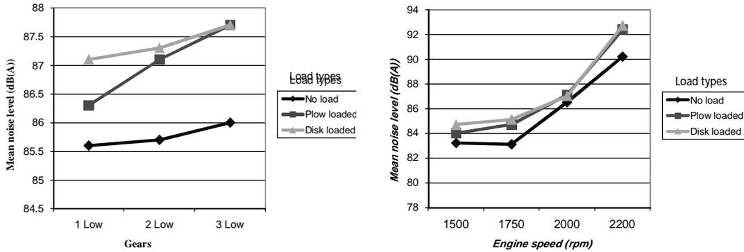
Figure 5. Mean noise level in different gears for tractor with open window cabin.
