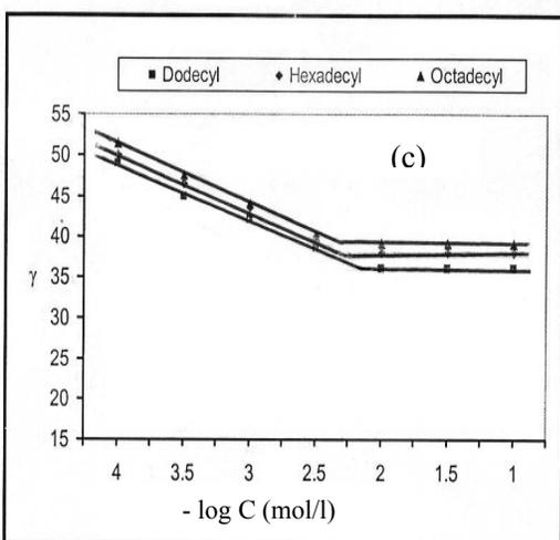
**Fig. 1 : Variation of Surface Tension ( $\gamma$ ) against Concentration of the Synthesized Schiff Base Amphiphiles at 25°C (a) SBA , (b) SBC and (c) SBS**
