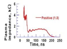
Figure 5. Time dependence of discharge impedance
