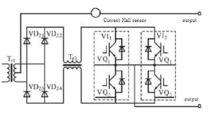
Figure 3. Second inverter circuit
