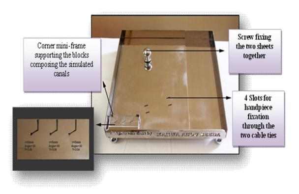
Figure 1: showing the cyclic fatigue testing device designed and made for the study, the lower left figure showing one of the two blocks used in this study
