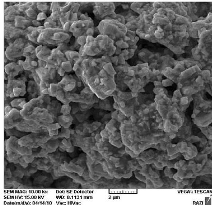
Fig.4: SEM topography coating surface
