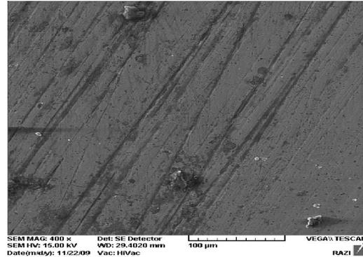
Fig 2: SEM topography of worn shaft surface
