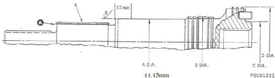
Fig. 1: Gas compressor shaft (subjected workpiece)
