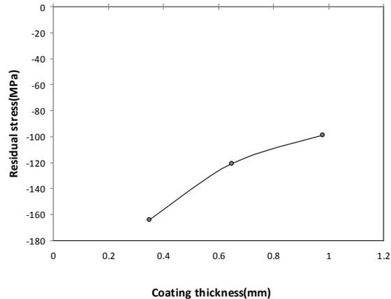
Fig.6: Compressive Residual stress from curvature method
