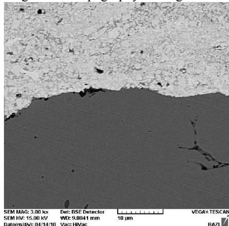
Fig.5: SEM micrograph of substrate-coating interface
