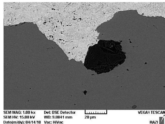
Fig.8: SEM micrograph a sand particle at the interface
