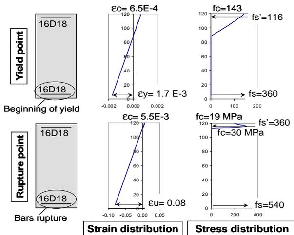
Fig. 13 Section analysis for yield and rupture points
