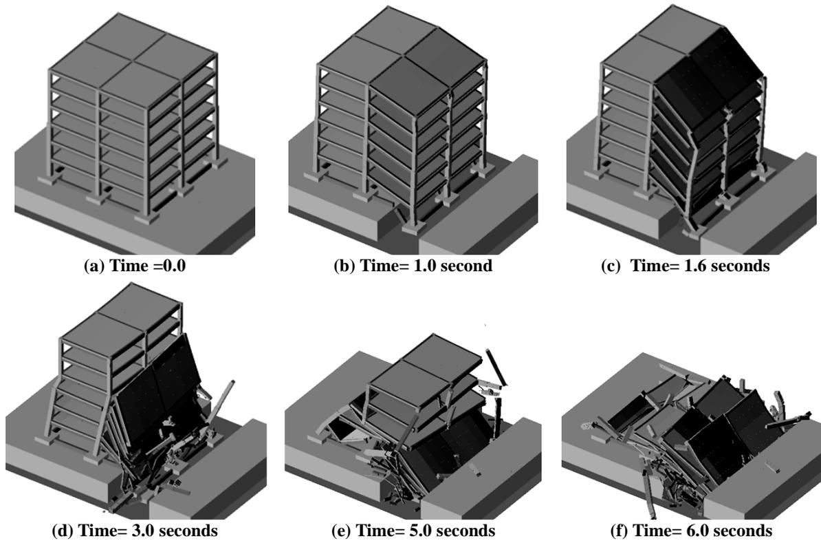
Fig. 5 Numerically-obtained progressive collapse for reference case (Org)
