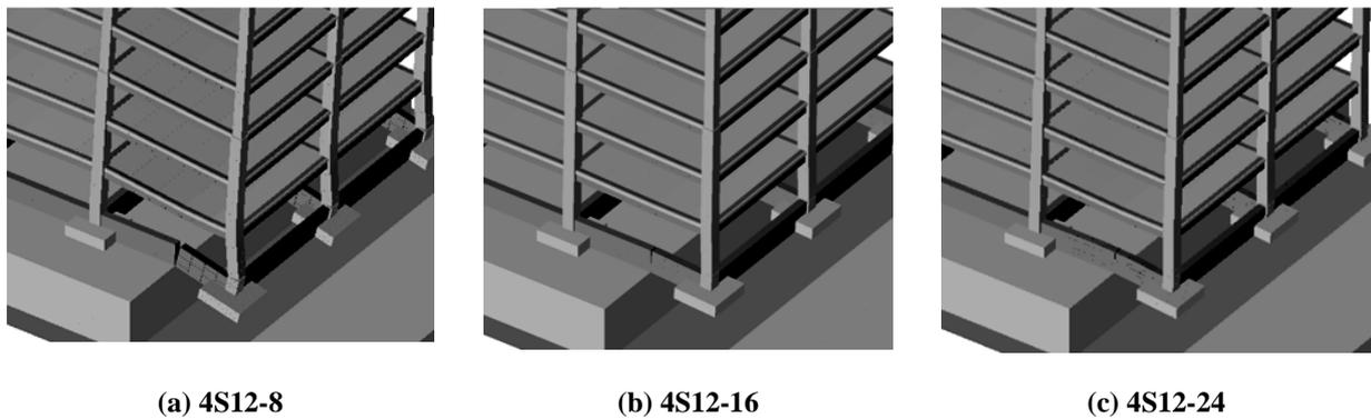
Fig. 9 Structural deformation (ten times magnified) for the structures with rigid tie beams
