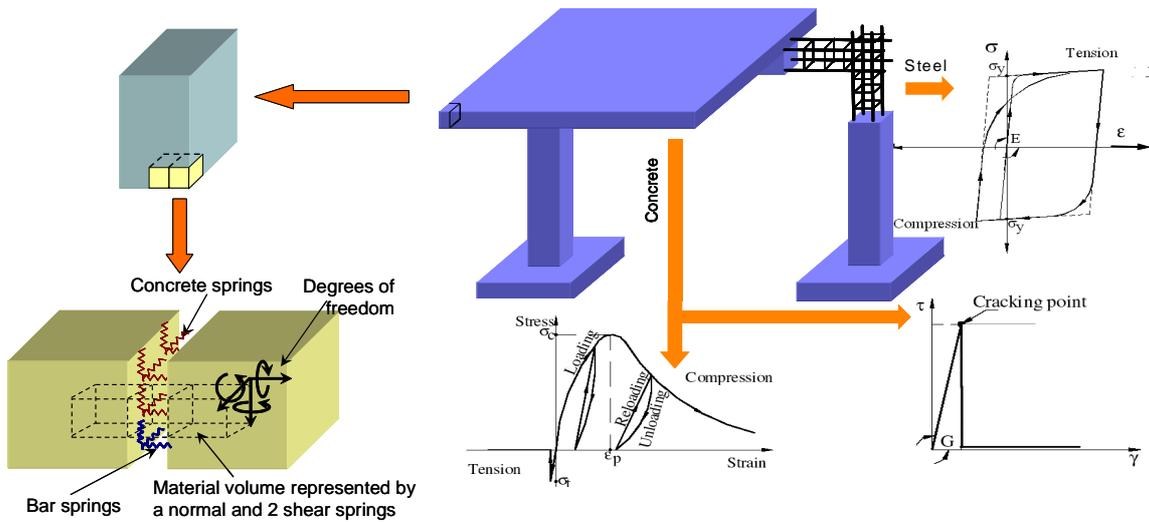
**Fig. 2 Modeling of a structure with the AEM**
