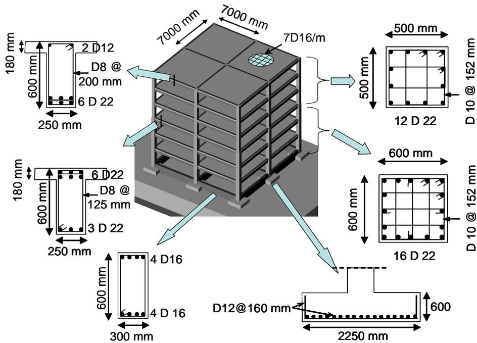
**Fig. 4 Details of the multi-storey framed reinforced concrete structure**
