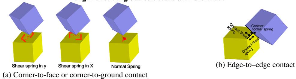
**Fig. 3 Different types of elements contact**
