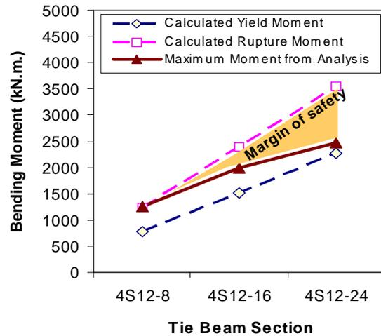
Fig. 14 Effect of reinforcement ratio on the capacity of tie beams
