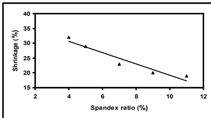
Figure 3: effect of spandex ratio on fabric shrinkage
