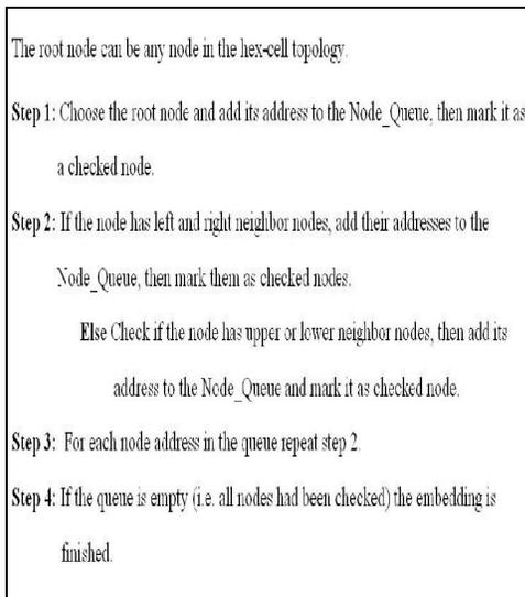
Figure 3: Embedding binary tree into hex-cell network
