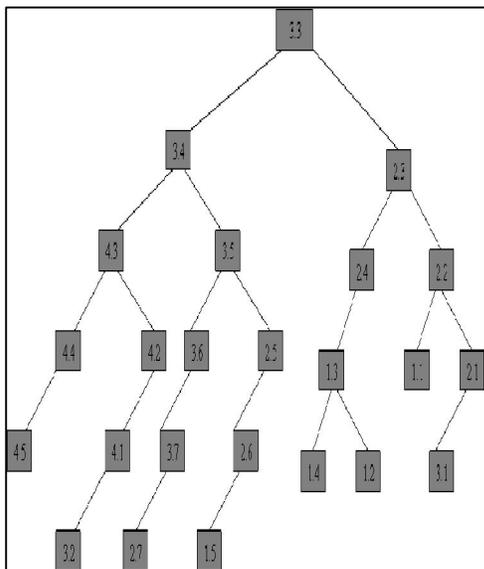
Figure 6: Embedding binary tree into hex-cell network
