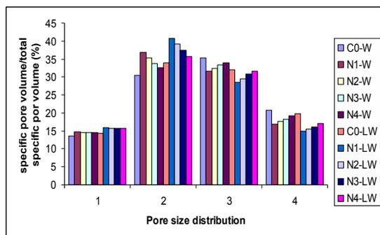
Fig. 2. Percent of specific pore volume of various grade pore size accounting for total specific pore volume.
