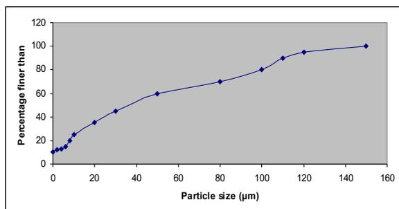
Fig. 1. Illustration of cement particles' distribution.
