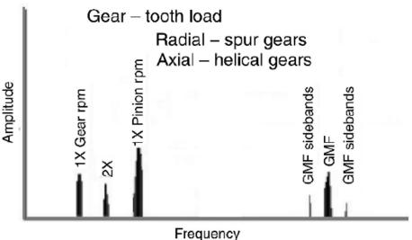
Fig 4- Gear tooth load
