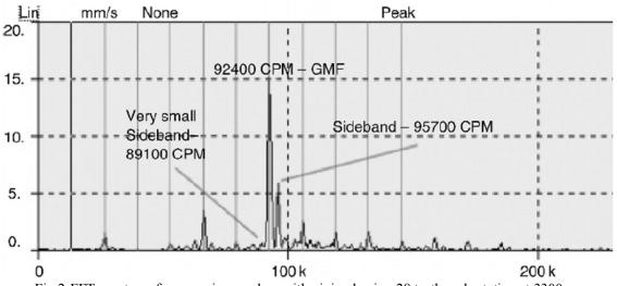
Fig 2-FFT spectrum from a noisy gearbox with pinion having 28 teeth and rotating at 3300 rpm
