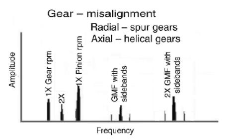
Fig 6-Gear misalignment
