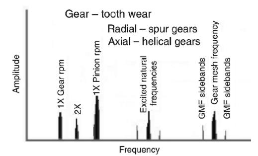
Fig 3-Gear tooth wear
