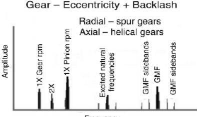
Frequency Fig 5-Gear eccentricity and backlash
