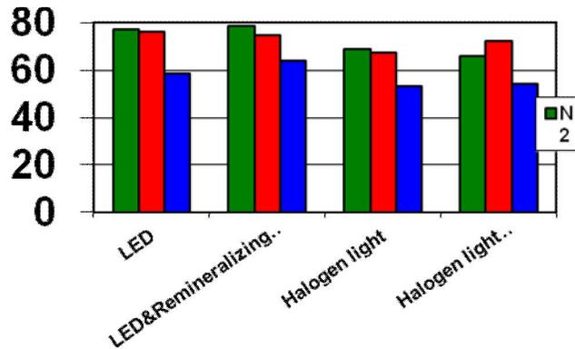
Fig. (1) Microhardness in different materials using different curing techniques at the top surface
