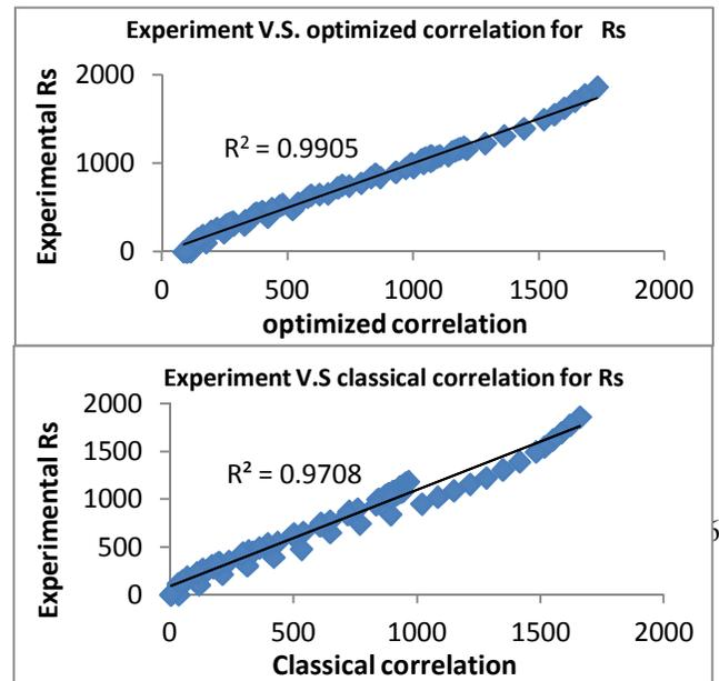
Figure (2): Regression analysis for solution gas-oil ratio
