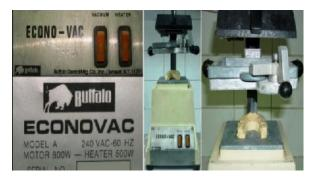
Fig.1: Vacuum former, pressure molding device with fabricated Night Guard over Patient cast
