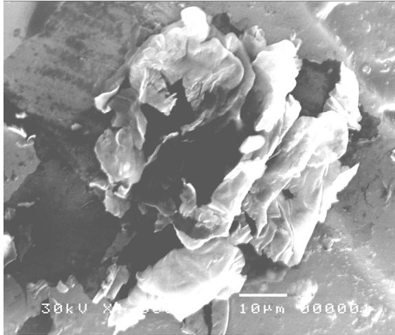
**Figure (5)** SEM micrograph of G1 after corrosion and irradiation with (10 kGy).
