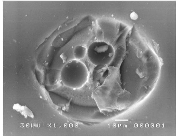
**Figure (9)** SEM micrograph of G2 after corrosion and irradiation with (100 kGy)
