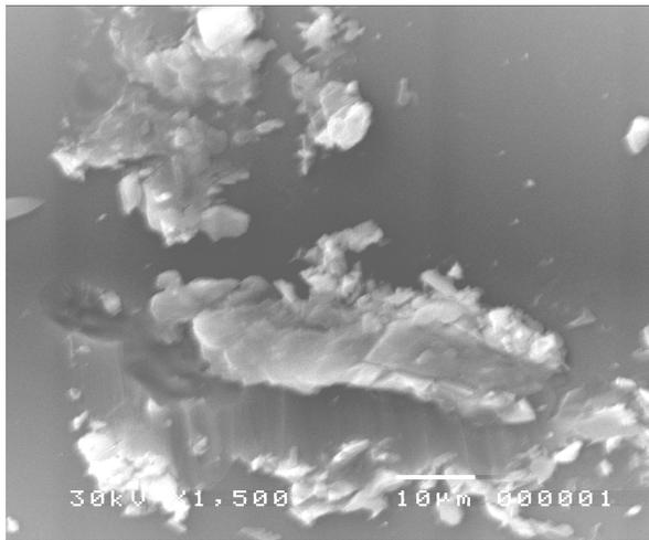
**Figure (6)** SEM micrograph of G1 after corrosion and irradiation with (100 kGy).
