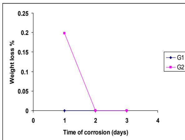
**Figure (3)** Weight loss % of nuclear waste glass (G1) & (G2) immersed in 0.5 N (NaOH) .
