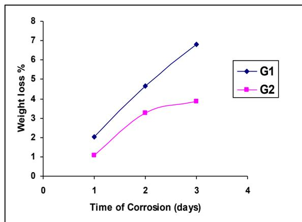
**Figure (2)** weight loss % of nuclear waste glass (G1) & (G2) immersed in 0.5 N HCl after gamma irradiation with 100 kGy.
