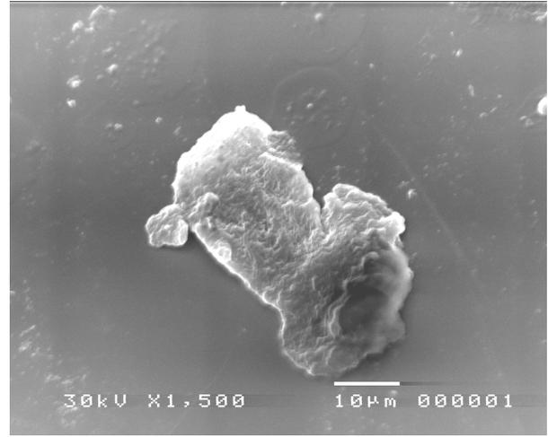
**Figure (8)** SEM micrograph of G2 after corrosion and irradiation with (10 kGy).
