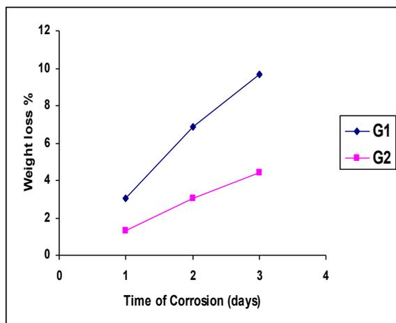
**Figure (1)** Weight loss % of nuclear waste glass (G1) & (G2) immersed in 0.5 N HCl.
