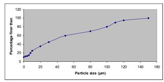
Fig.1. Particles distribution pattern of ordinary Portland cement.
