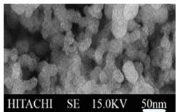
Fig. 2. SEM micrograph of SiO<sub>2</sub> nanoparticles.
