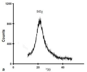
Fig. 3. XRD analysis of SiO<sub>2</sub> nanoparticles.
