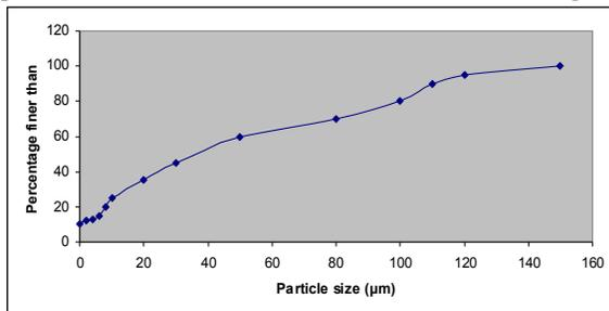
Fig. 1. Particles distribution pattern of ordinary Portland cement.
