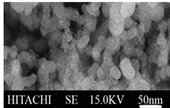
Fig. 2. SEM micrograph of SiO<sub>2</sub> nanoparticles.
