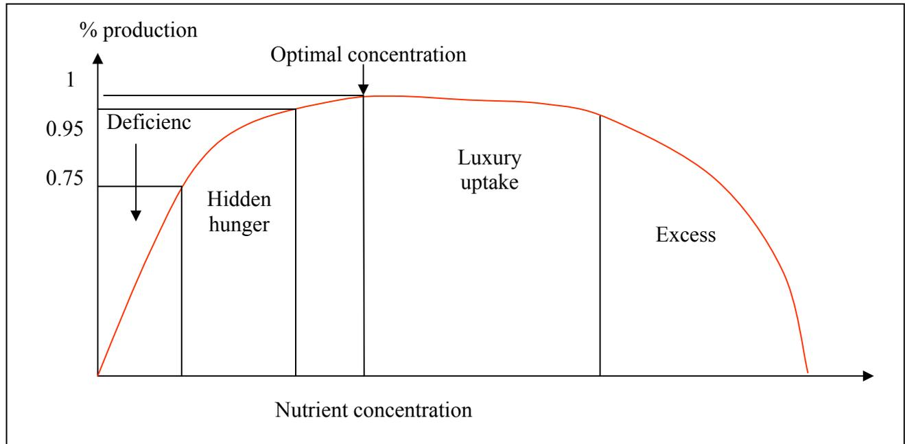
Fig. 1: graphical representation of the production ranges crossed increasing the concentration of a nutrient (modified after Schulte and Kelling, 1986).
